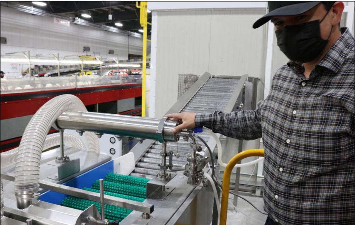
Ricardo Rivera, Apeel Sciences, demonstrates where the cucumbers are sprayed on the conveyor belt before entering the drying chamber.
