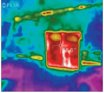
Photo 1. Infrared photo taken with a Flir camera—shows warmer surface of the door and leakage around the doors.
