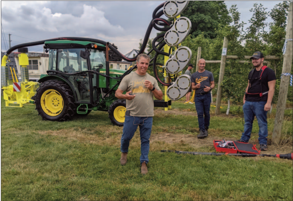
Joe Pillitteri, president, Lakeview Vineyard Equipment, demonstrates the leaf remover for apple orchards.
