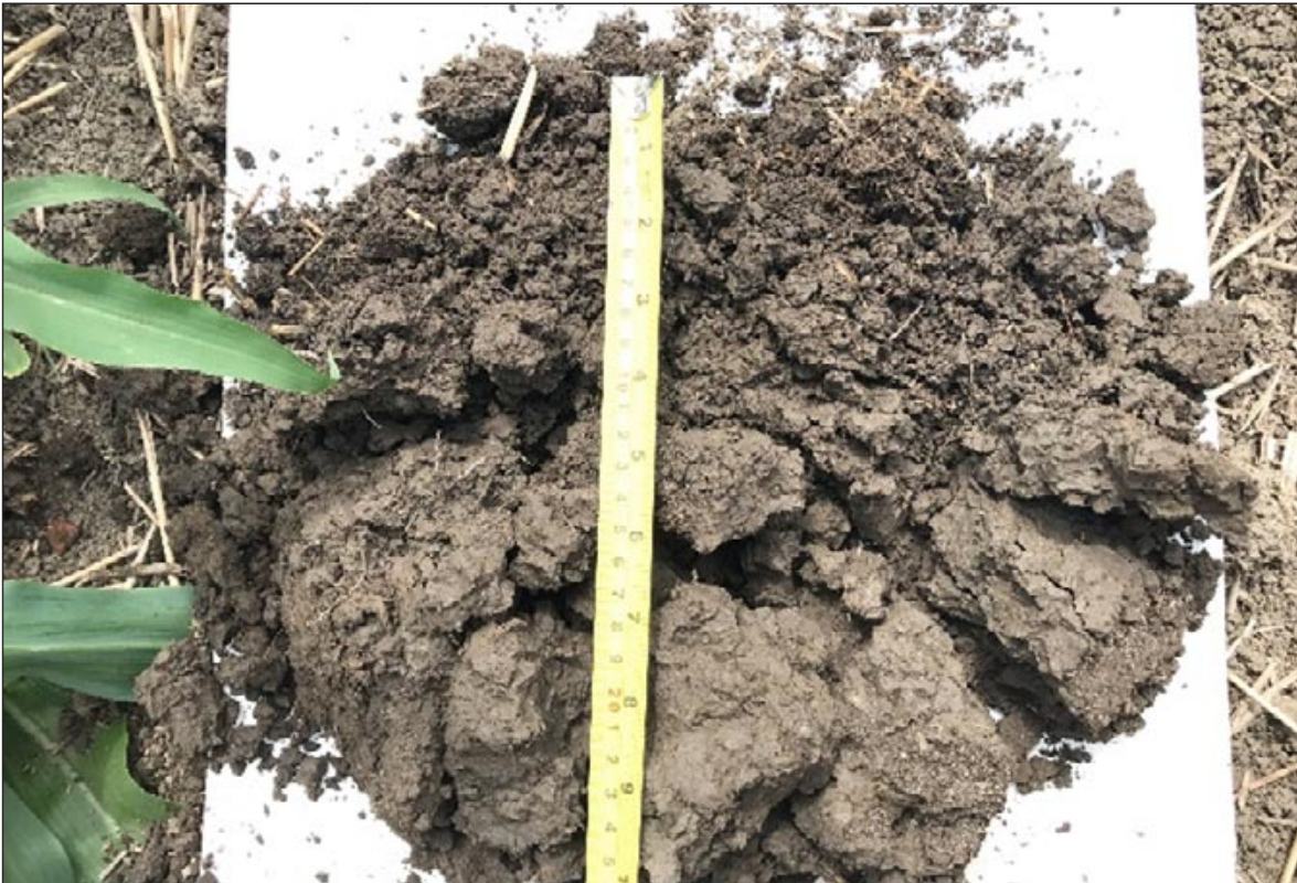
Figure 4. An example of a soil being evaluated using the visual evaluation of soil structure (VESS) within the soil structure assessment module.
