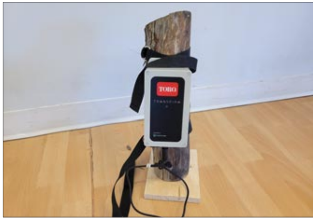
Toro Transpira measures plant water consumption by direct plant sensing.
